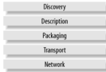
Figure 1-5. The web service technology stack
