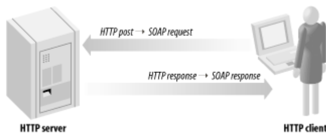
Figure 2-5. SOAP request messages are posted to the HTTP server and response messages are returned over the same HTTP connection
